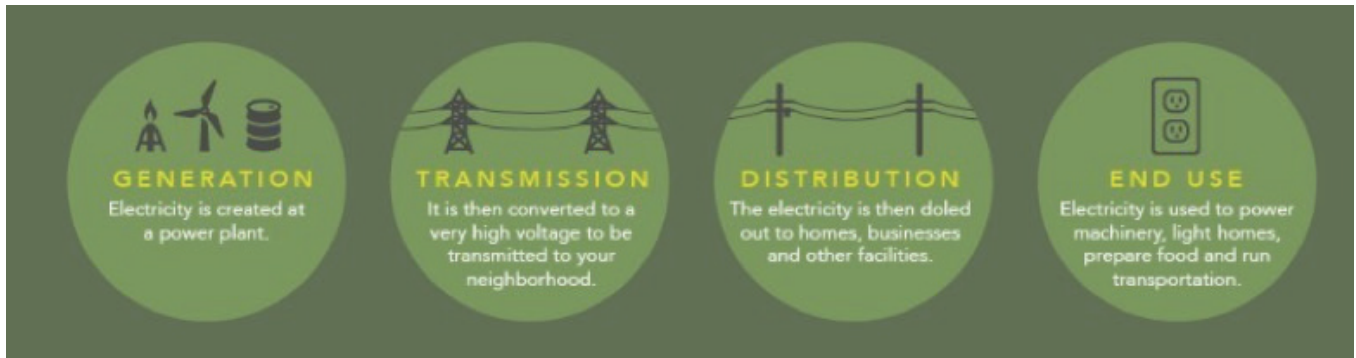
FIGURE 1. ELECTRIC POWER GRID
